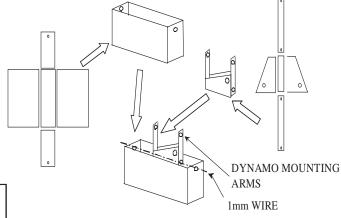
The next step uses the etched V hangers differently on the Pullmans to the way they were intended initial kits only.
