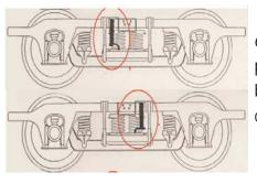
61) Affix the dampers into place as shown left noting that the bottom mounting faces towards the centre in both cases.
