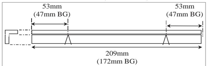
25) Cut 2 lengths of angle truss moulding 209mm (172mm for BGs) and make a notch in one side of the angle 53mm (47mm for BGs) from each end (see diagram right) - a simple cut with a
