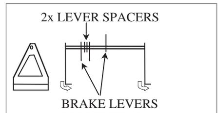
35) Attach to the central brake lever a pull-rod and adjuster that would actually pull the bogie brake gear (see right). The pull-rod length should be trimmed to length just forward of the inner axle of the adjacent bogie.
