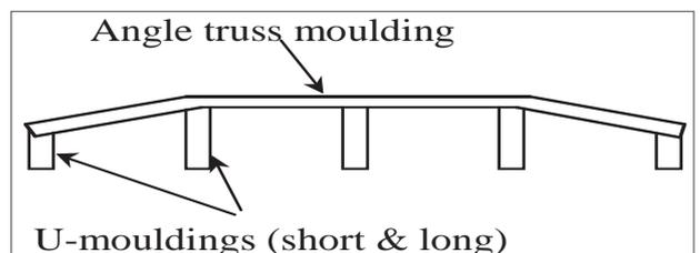
the edges of the shorts 'U' mouldings. Allow the solvent to harden on the centre 'U' mouldings before attaching the ends to the short 'U' mouldings as these may need bending a little more to achieve good alignment of the parts. The top of the angle should be level with the tops of the 'U' shaped mouldings.
