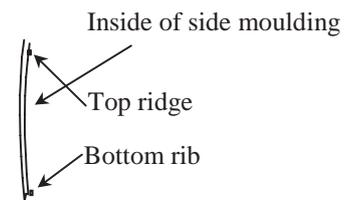
3) If constructing a brake vehicle the guard's doors require the bottoms modifying. They are depicted by removing the bottom of the door level with the bottom of the lip moulded on the inside of the body to the full width of the door opening. Start by cutting (with a fine razor saw) up the door scribe marks, about 1.5mm max., then remove the material between the two cuts (see right).
