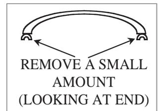
16) Take an end moulding and check the fit of the underside of the roof to the curved top of the end. The two parts should sit snugly together, if not check the areas shown in the diagram (right) and carefully trim away just sufficient material to allow the parts to meet. The roof moulding sits over the top of the end moulding with an overhang of about 1mm at the gutter
