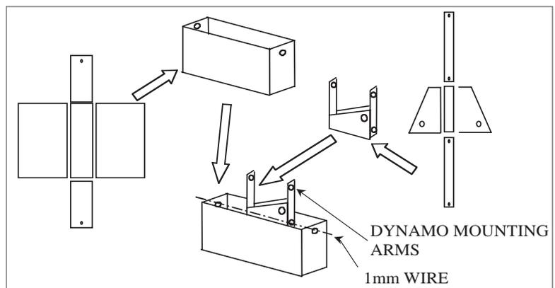
54) Remove the Regulator Carrier Frame (E9) from the etch and fold along the half etches to form a U-shaped bracket. Fold in the fuse box mounting plate (away from half etch) and mount the cast metal regulator box (C22) and fuse box (C19) as shown right (see photos on our CD).
