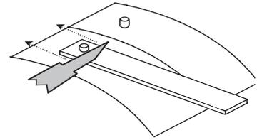
8) This vehicle has frameless windows, so check that they will fit in the openings. Occasionally some openings can be a little too tight for a good fit after the sides have been painted. Make any adjustments to the windows NOT the openings.
