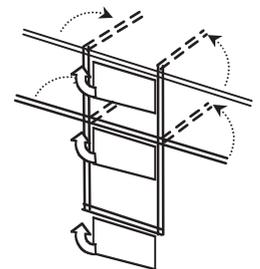
**27.16)** To mount the steps, drill four small holes in the bogie sideframe (0.6mm), the top two are directly under the top channel of the bogie and positioned so that the steps are about 1mm from the edge of the centre bolster detail. (See photographs on disk)
