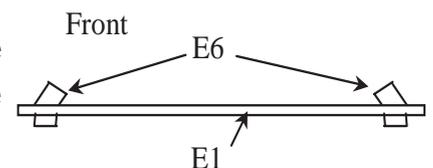
17) Decide which type of windscreen wipers you are to fit and drill out the mounting holes 0.4mm (half etched dimples above and below the window openings). Single arm wipers have a single hole below the window and the double arm type has two holes above the window - DO NOT FIT THE WIPERS YET.
