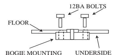
**33)** Fit the floor in place and drill 2x 1.8mm holes at each end through the floor and the body stretchers about 6mm from the end and 8mm from the sides. Also drill a 4mm hole in line with the toilet window opening and centrally across the floor width (See underframe layout for position). This will be used to support the floor with a long bolt up into the previously fitted roof captive nut. Adjust nut position accordingly.
