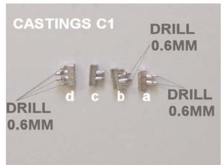
43.3) Fit the castings to the underside of the bufferbeams centrally under each buffer as follows when looking end on: C1d cab left, C1c cab right, C1b non-cab left, C1a non-cab right. Remember you'll be working upside down so it's easy to get the order wrong! Since the rear bufferbeam is attached to the underfloor you might wish to leave them until you're adding those details, but if you do don't forget about them.
