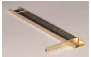
28.16) Glue the bogie channels to the front and rear of each bogie with the bottom of the channel level with the bottom of the sideframe (superglue is recommended for this). The arrangement of these channels should be:
