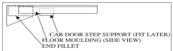
*\*\*TIP - it may be prudent to back the end fillet with scrap styrene to improve its robustness as shown dotted in the diagram.*
