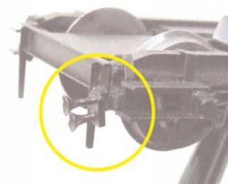
the bogie front against the guard iron. If you opt to do this, reduce the length of the mounting bar to just above the first horn and butt it up to the bottom of the front channel.
