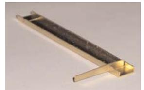
38) Fold up the bogie step tread supports and mounting brackets (E2). See Bogie step and speedo drive.jpeg
