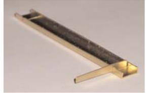
25.16) Glue one each of the bogie channels to the front and rear of each bogie with the bottom of the channel level with the bottom of the sideframe end (superglue is recommended for this). The guard irons go to the front of the bogie in each case (the motor is at the rear of the power bogie). See also Bogie end channel in place.
