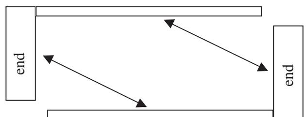
each other) your sides will be level at the bottom. Ensure the outside faces of the sides are a good match, in profile, to the outside of the ends at the door line.
