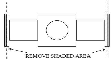
25.2) Push brass bearings into the axle holes making sure they are an easy sliding fit, but not sloppy - if necessary clean hole with a 2.5mm drill. Do not fix in position as adjustments will be made later.
