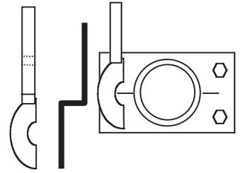
40) Drill two 1.8mm holes in the bufferbeam at the guard end only to accept the exhaust pipes. The holes should be 4mm in from the edge of the buffer mounting pad and hard against the underside of the cab floor (left hand side only shown).
