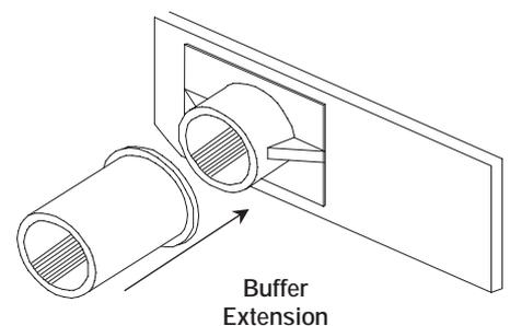
38) Install the floor into the body and temporarily secure into position. Now fit the bufferbeams to the underside of the cab ends, aligned centrally across the cab and butted firmly against the ends of the extended solebars to ensure vertical squareness. **DO NOT GLUE THE BUFFERBEAM TO THE SOLEBAR EXTENSIONS AS THIS WILL ALSO PREVENT THE FLOOR FROM BEING REMOVED.**
