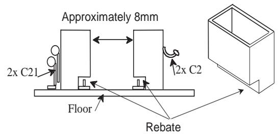
49.9) Add 2 fillers C2 to one tank as shown in the diagram, they should be positioned (vertically) so that the filler caps are just below the solebar. Prototype photo: Exhaust And Radiator.JPG
