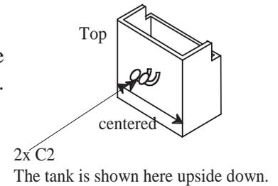
49.10) Affix the two piggy-backed air tanks (C21) to the other fuel tank, again cantered and positioned level with the top of the fuel tank as shown in the two diagrams here.
