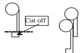
49.6) Cut and file the two small boxes from casting C8 and remove the mounting foot from the rear. This will leave you with (mainly) a single large box with a flat mounting, see right.
