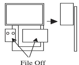
49.7) Cut the pipe extensions off the exhaust silencers C9 as shown right.
