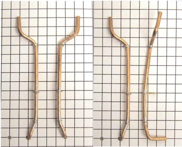
The 122 stacks do not have the top bends as shown here (left), but simply go straight up either side of the small destination box.
