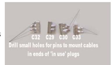
43.2) Drill a small hole in the castings (0.6mm) just deep enough to secure a short length of wire. Insert short pieces of wire leaving about 3mm protruding onto which the cable sleeve will be fixed. On part C32 there are four holes to be drilled because the cables are depicted as stowed so form a pair of loops.
