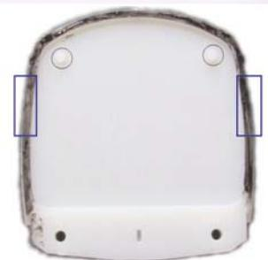
23) With a fine razor saw, cut off the moulded on bufferbeam level with the bottom of the end. Use the underside of the end as a fence to guide the saw blade and finish off with a flat file to remove any burrs.
