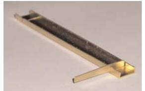
27.16) Glue the bogie channels to the front and rear of each bogie with the bottom of the channel level with the bottom of the sideframe (superglue is recommended for this). The arrangement of these channels should be:
