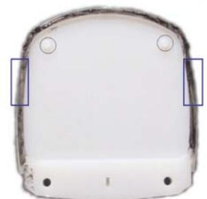
16) With a fine razor saw, cut off the molded on buffer beams level with the bottom of the ends. Use the underside of the end as a fence to guide the saw blade and finish off with a flat file to remove any burrs.
