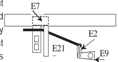
37) Cut a short length of brake shaft material and make sure it will slide into the handbrake pivot hole. Insert the brake arm E21 into the pivot hanger so that the longest part of the arm is facing to the right and insert the short pivot just made.
