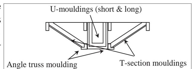
18) To add additional rigidity to the floor we have included an etched rib that you could put in place now. Remove part E27 and smooth off the burrs and fold it along the half-etched line until it will
