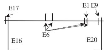
32) Attach the brake hanger assemblies to the floor with E18 to the outside - see underframe diagram for positions. Now thread the brake vac cylinder into place so that the outer mounting is inside the V of the hanger and to the left of the brake shaft, i.e. on the opposite side of the shaft to the bogie, secure in place. See image Brake Hanger.jpg
