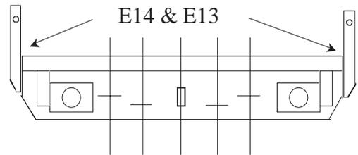
54) Test fit the end doors between the quarter pillars, and then attach the doors to the floor keeping everything flush and upright - there may well be a small gap between the doors and pillars, just equalise this each side.
