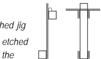
*Since it is essential to get the handrails straight, we have created an etched jig to assist (E10 - two actually). To use this fold the tabs 90° towards the etched fold lines and affix a short length the handrail wire (about 40mm) across the top. To use, simply press the jig against the solebar with the bottom tabs hard up against the underside. Now each handrail can be pressed gently against the underside of the wire to obtain the correct height.*
