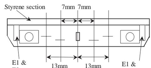
8) Cut two lengths of 1mm x 1.5mm styrene to the length of the top of the bufferbeam and affix to the top of the bufferbeam ensuring the widest dimension of the section is laid onto the molding and the front faces are flush. Sand flat both front and back as required. See above.
